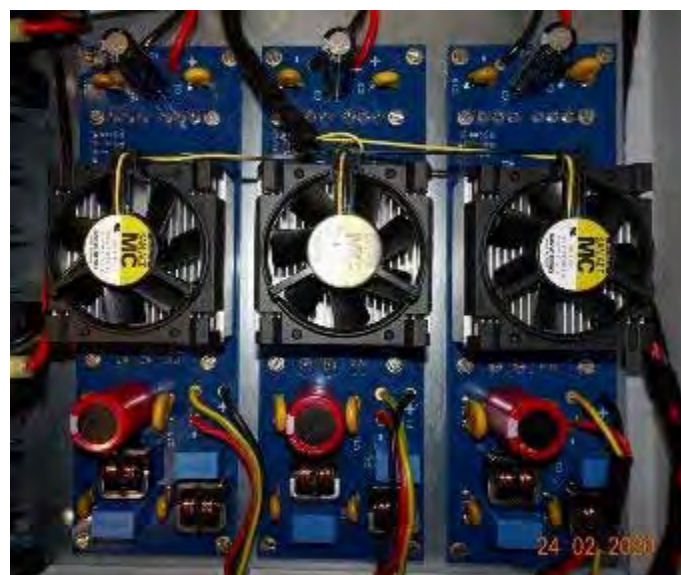
Figure 10: Heatsink with cooling fans
