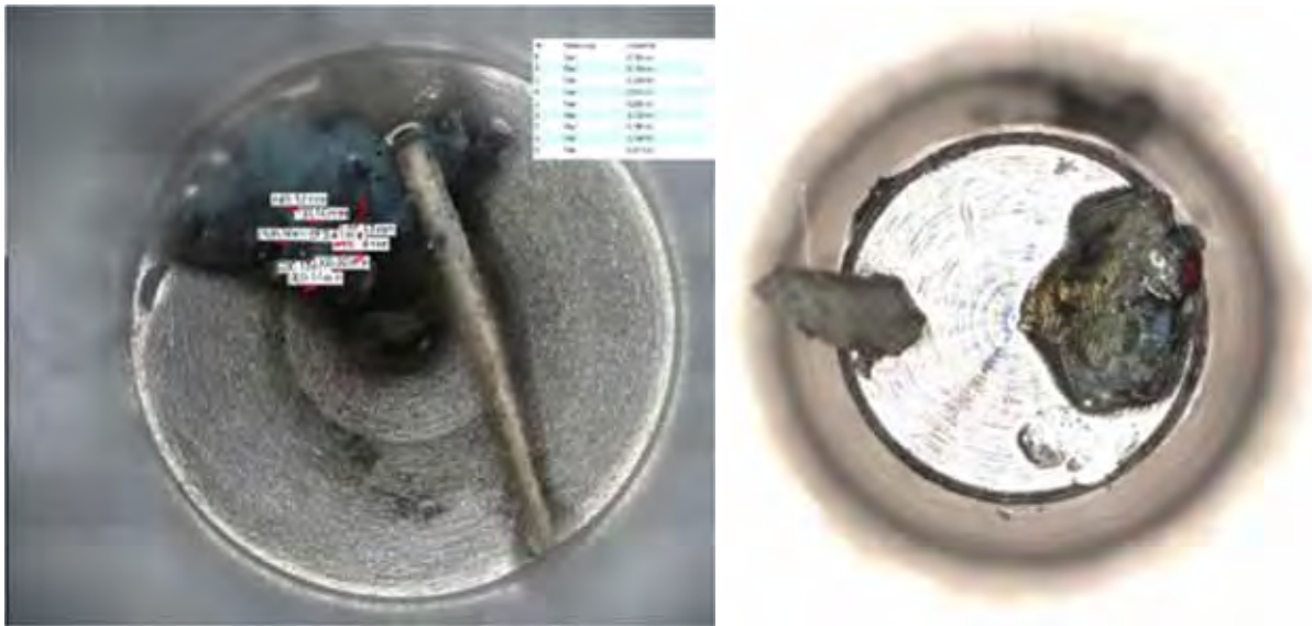
Figure 60: 2 nd failure of EXV no. 2 – particles in EXV no. 2
