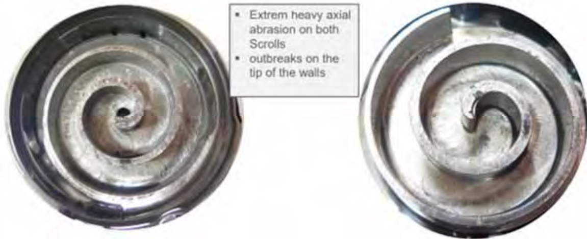
Figure 52: Compressor no. 1 - Scrolls after failure
