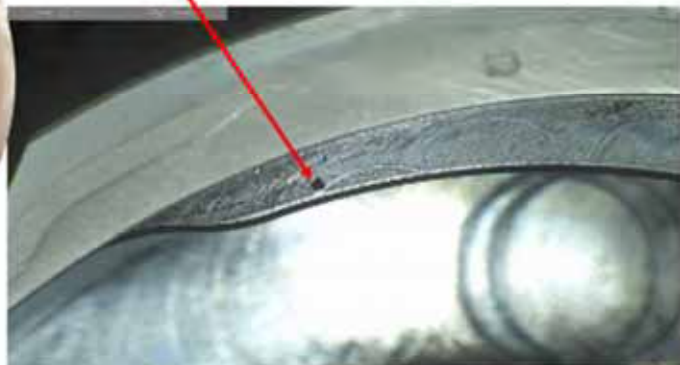
Figure 55: Compressor no. 2 – Indication for external particles at scroll inlet after 30 min operation
