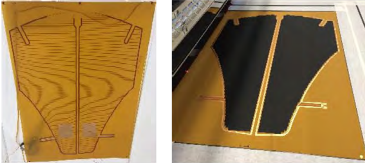
Figure 7: Substrate after etching- (left) and screen-printing process (right)
