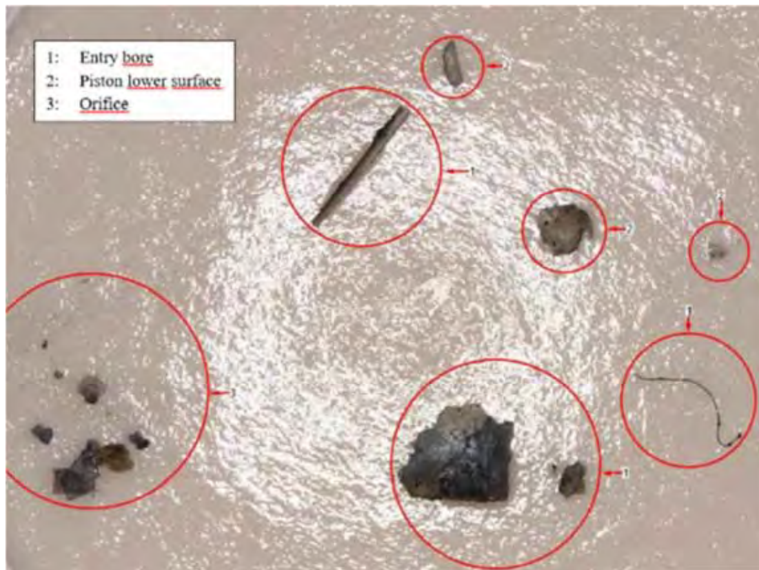
Figure 61: 2 nd failure of EXV no. 2 – particles found
