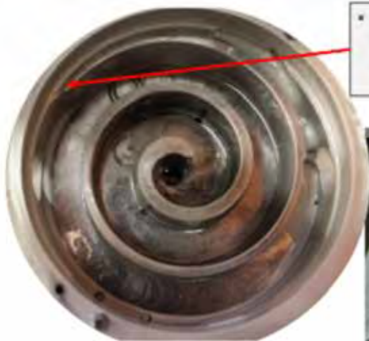
Figure 55: Compressor no. 2 – Indication for external particles at scroll inlet after 30 min operation
