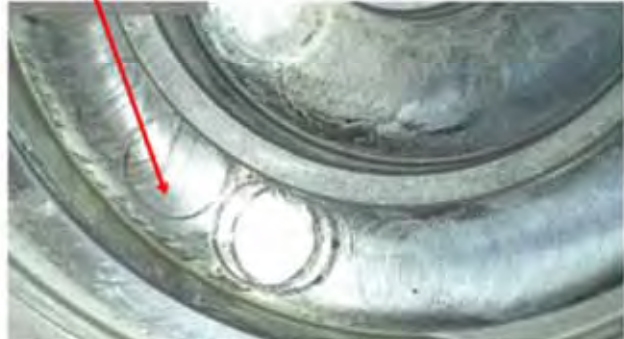
Figure 54: Compressor no. 2 – Wear marks at scroll after 30 min operation
