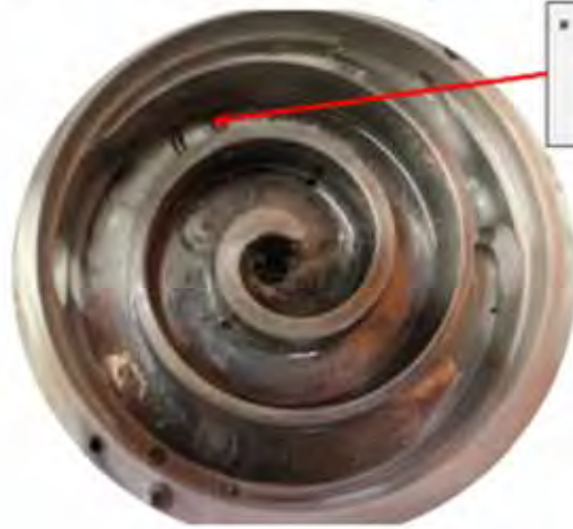
Figure 54: Compressor no. 2 – Wear marks at scroll after 30 min operation
