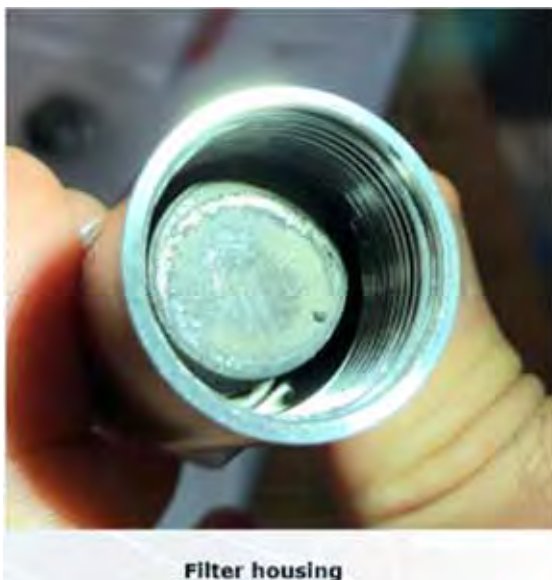
Figure 46: Contamination of the refrigerant filter after failure of compressor no. 1
