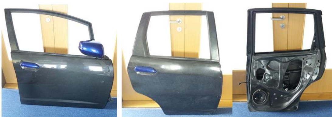
Figure 11: Manufactured lightweight composite front and rear side doors at ECON office
