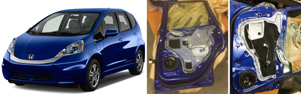
Figure 3: Original steel closures on a Honda Fit EV (left) and at the ECON workshop partially disassembled (two on the right)
